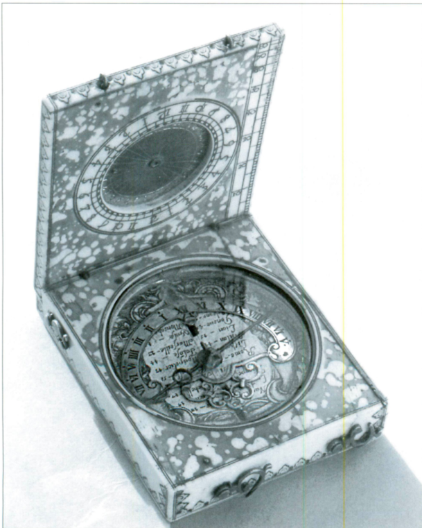
Fig. 1. Dieppe Magnetic Azimuth Dial with shadow of its lid exactly falling across its lower leaf.
